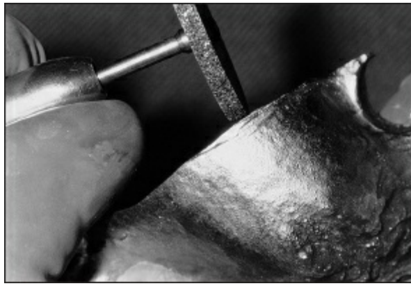
Fig 17-20 An overextended major connector may be shortened using a heatless stone in a low-speed handpiece or dental laboratory engine.
