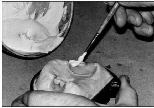
Fig 15-56 After the second investment layer has been coated with separating medium and soaked in supernatant dental slurry, the third investment layer is added. A stiff brush is used to paint stone around the necks of the artificial teeth and over the surface of the wax.
