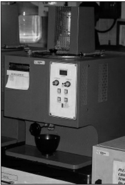
Fig 11-25 An automated duplicating machine is used in the preparation and storage of reversible hydrocolloid impression material.
