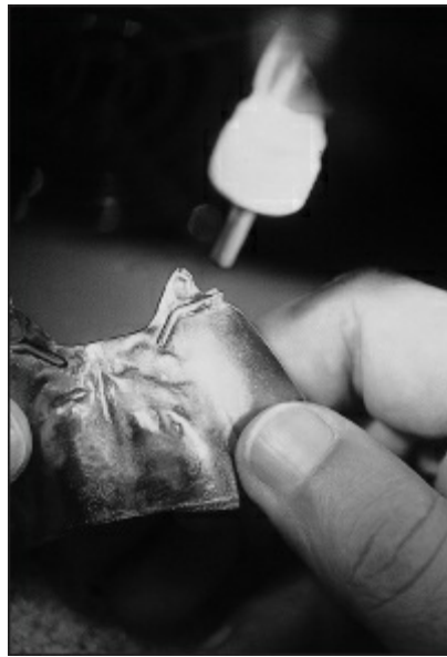
Fig 11-64 The framework is placed within the chamber of the laser welder. Welding occurs in an argon-rich environment, which improves the quality of the weld.
